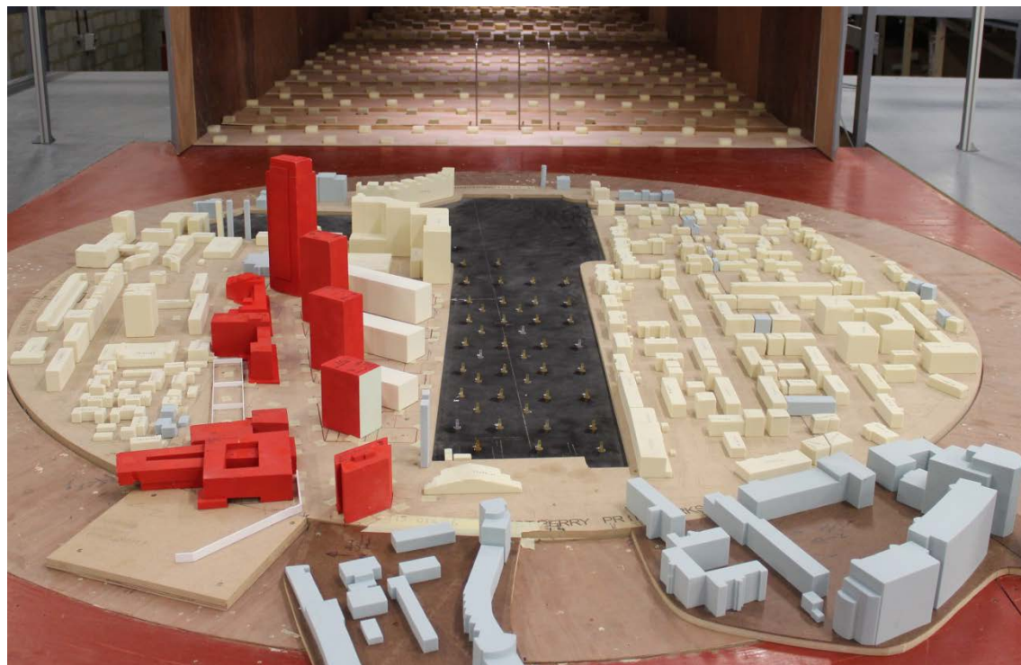
Figure 32: M5 - Option 5 (Blocks T01, T02, T03, T04 relocated and Blocks B02, B03 and B04 massing changed and relocated) with existing surrounding buildings – View in the wind tunnel (from the north and west)
