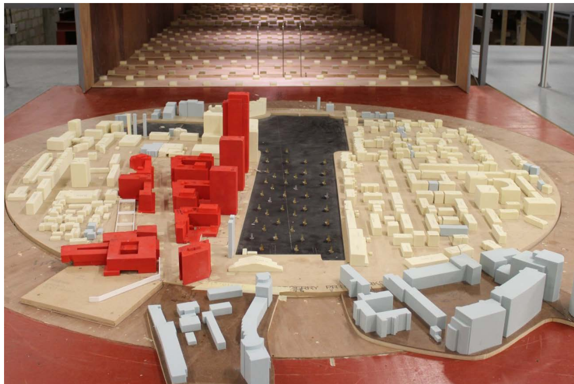
Figure 28: M1 - Option 1 (Block T01 removed) with existing surrounding buildings – View in the wind tunnel (from the north and west)
