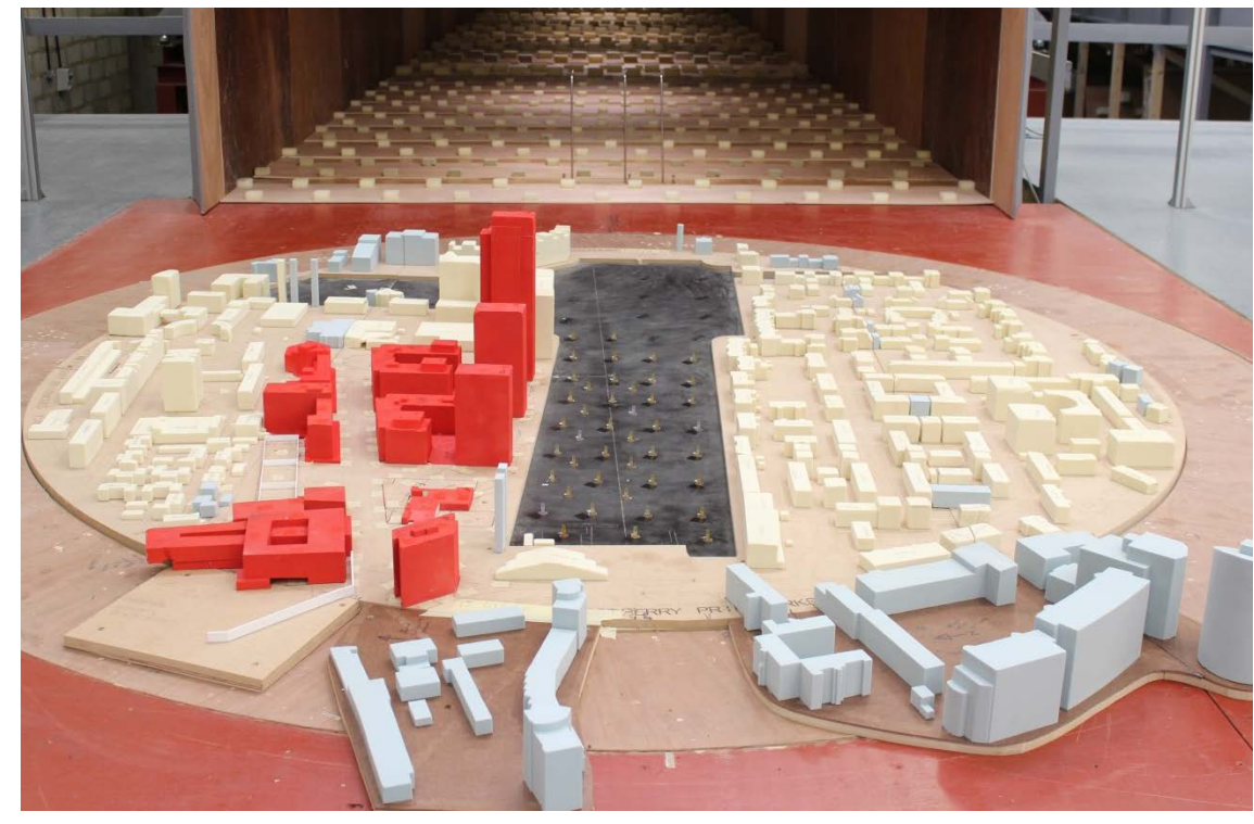
Figure 29: M2 - Option 2 (Blocks T01 and B02 removed) with existing surrounding buildings– View in the wind tunnel (from the north and west)
