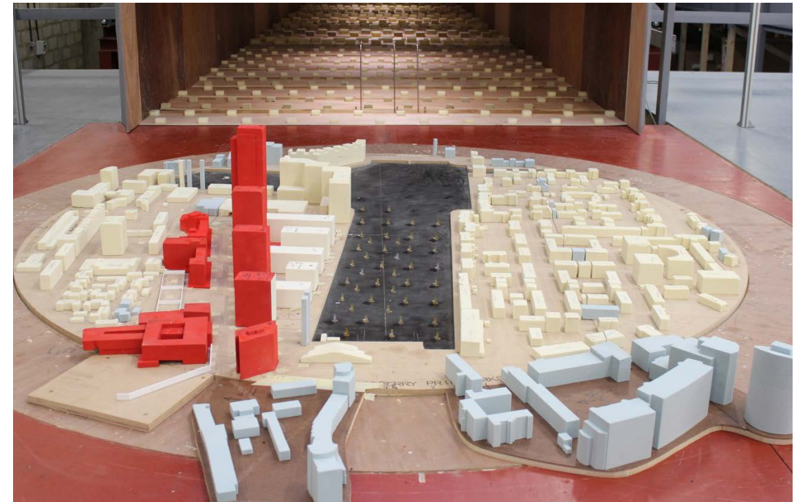
Figure 31: M4 - Option 4 (Blocks T01, T02, T03, T04 relocated and Blocks B02, B03 and B04 massing changed) with existing surrounding buildings – View in the wind tunnel (from the north and west)
