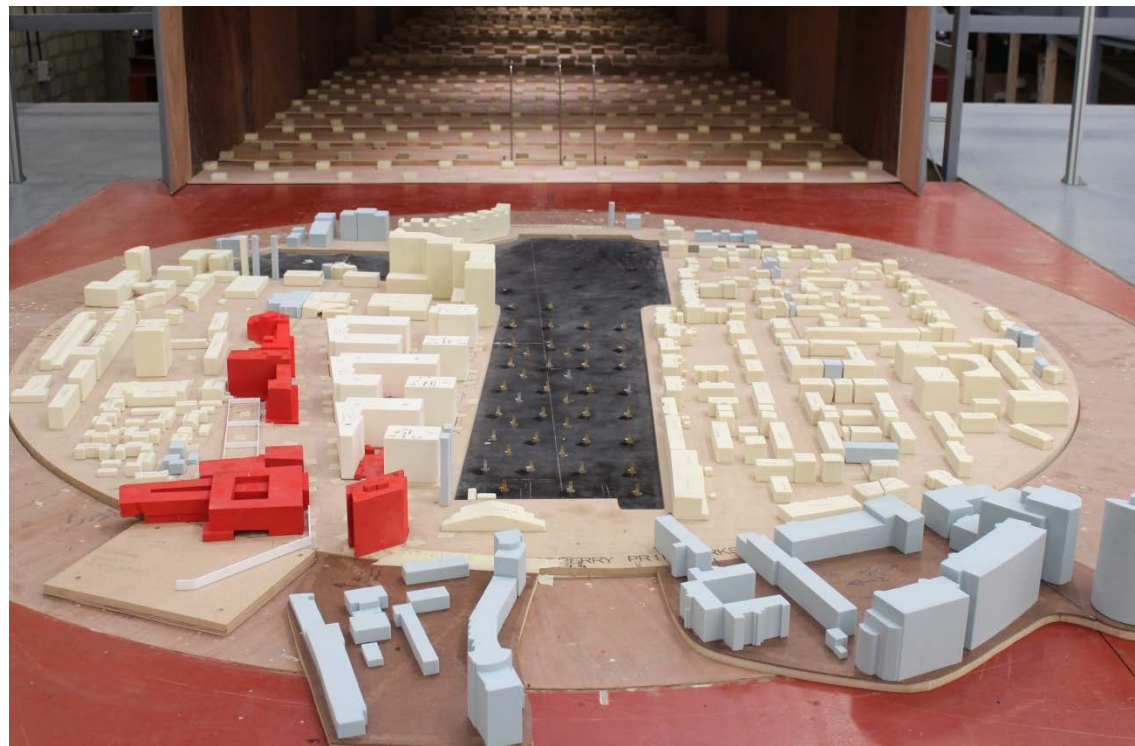
Figure 30: M3 - Option 3 (Blocks T01, T02, T03, T04, B02, B03 and B04 height reduced to 25m) with existing surrounding buildings – View in the wind tunnel (from the north and west)
