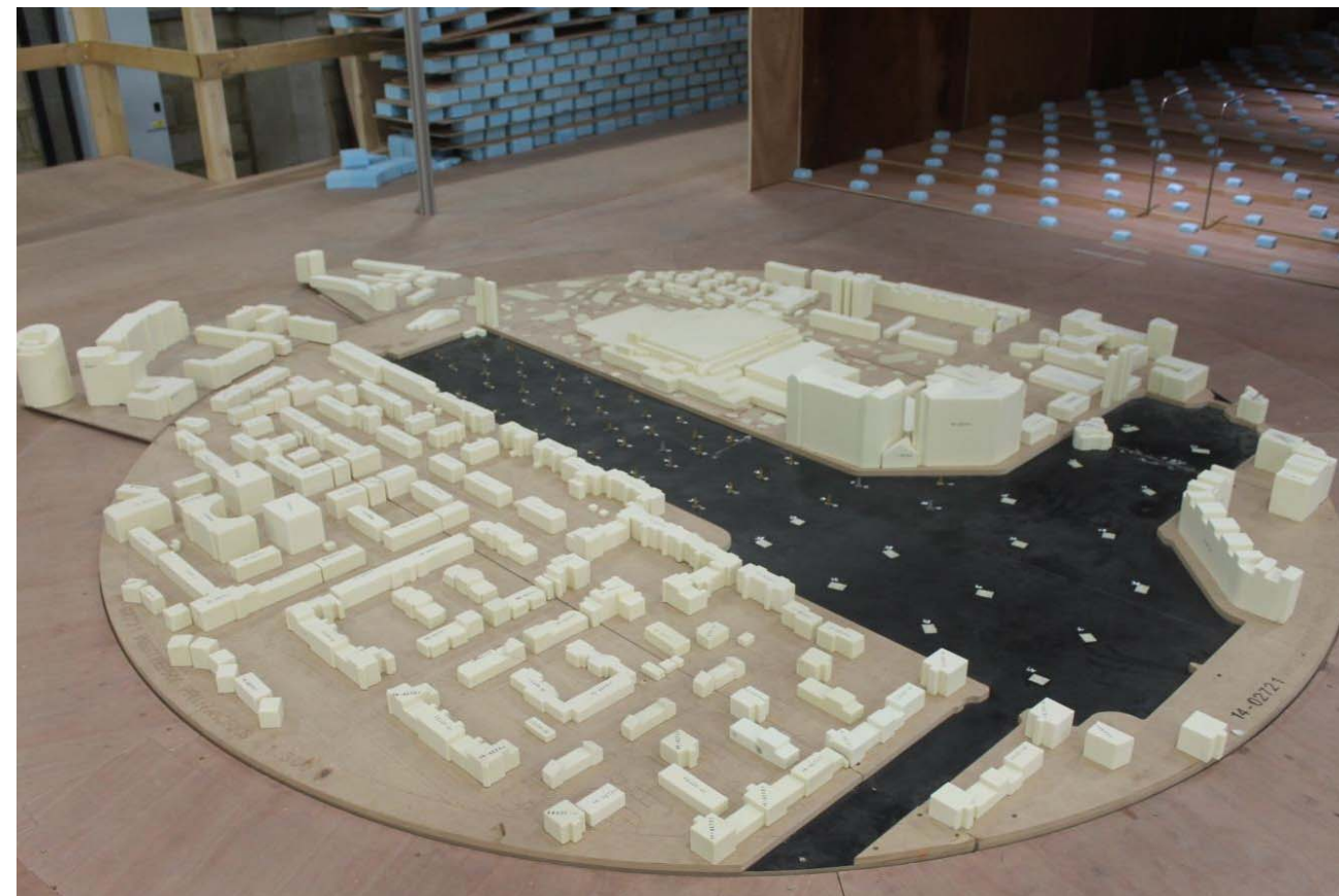
Figure 17.2: Wind Tunnel test Model for the Development
