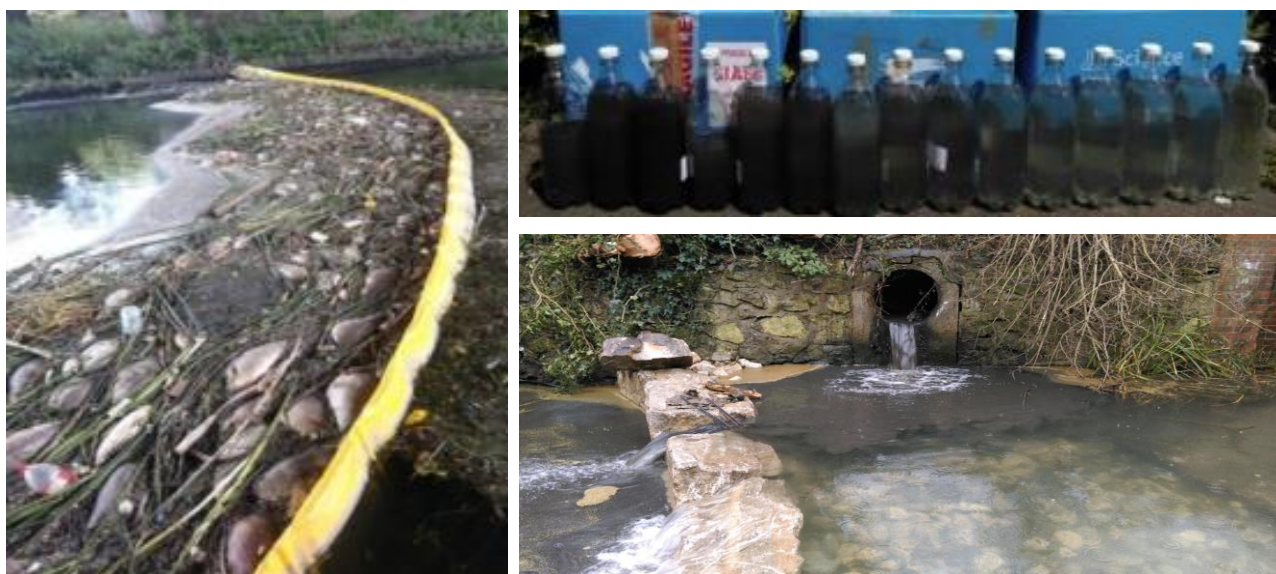
Figure 1 – (clockwise) A fish kill on the River Lea, Olympic Park, Aug 2013 caused by road runoff; Water samples taken every 15mins during a rainfall event; and Road runoff entering the Hogsmill River
