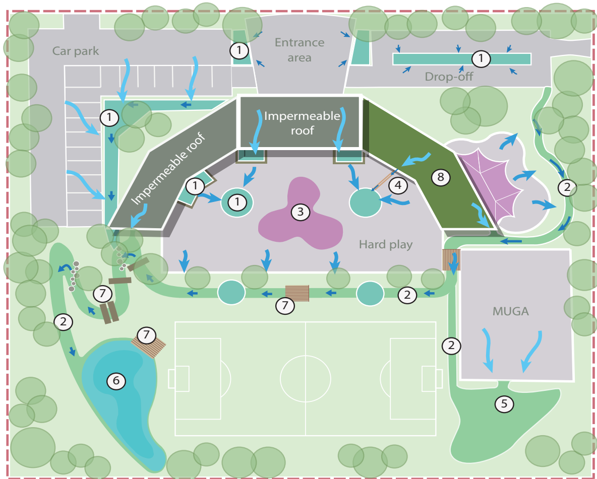
Figure 2.11 Concept for retrofitting SuDS
