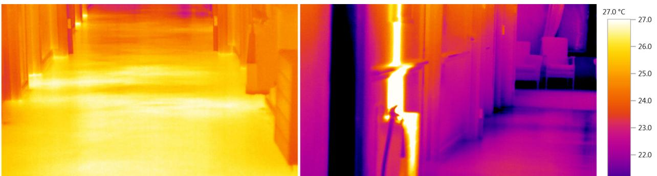
**Figure 7. Thermal imaging showing a distinct floor temperature difference between the first floor corridor (left) and the second floor corridor (right)**
