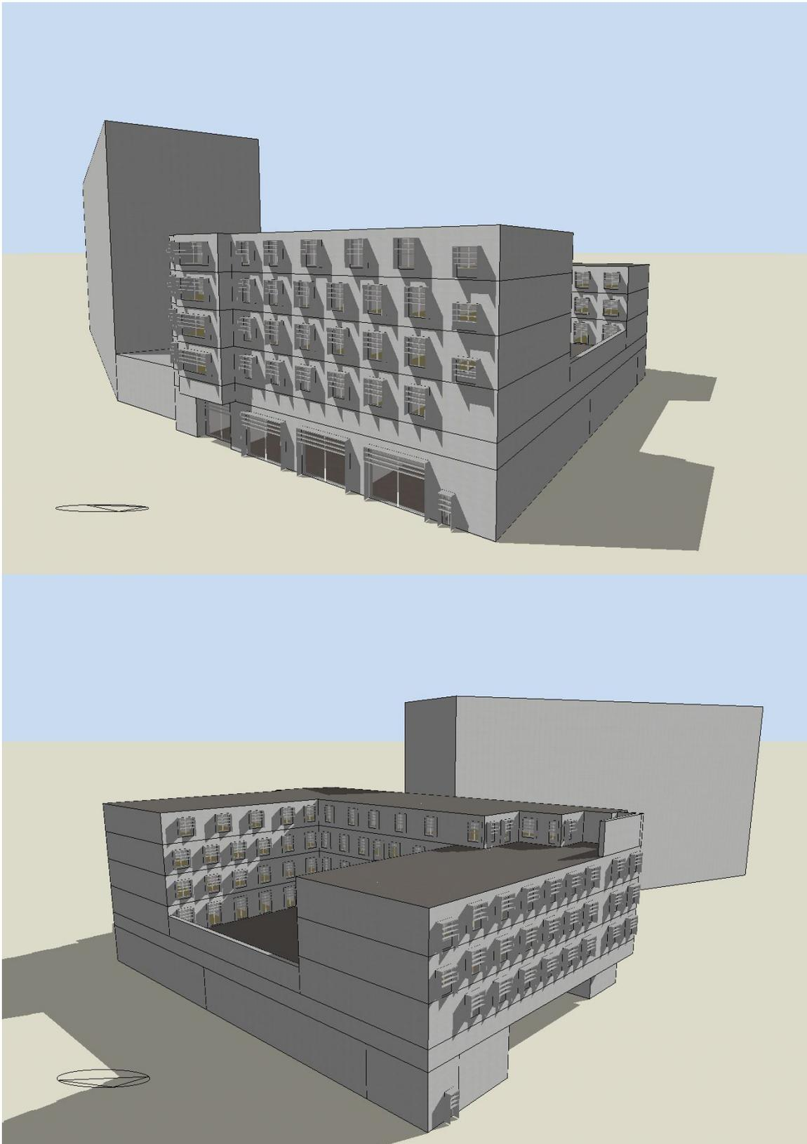
**Figure A 2. Rendered views of the DesignBuilder model incorporating external window louvres and side fins**
