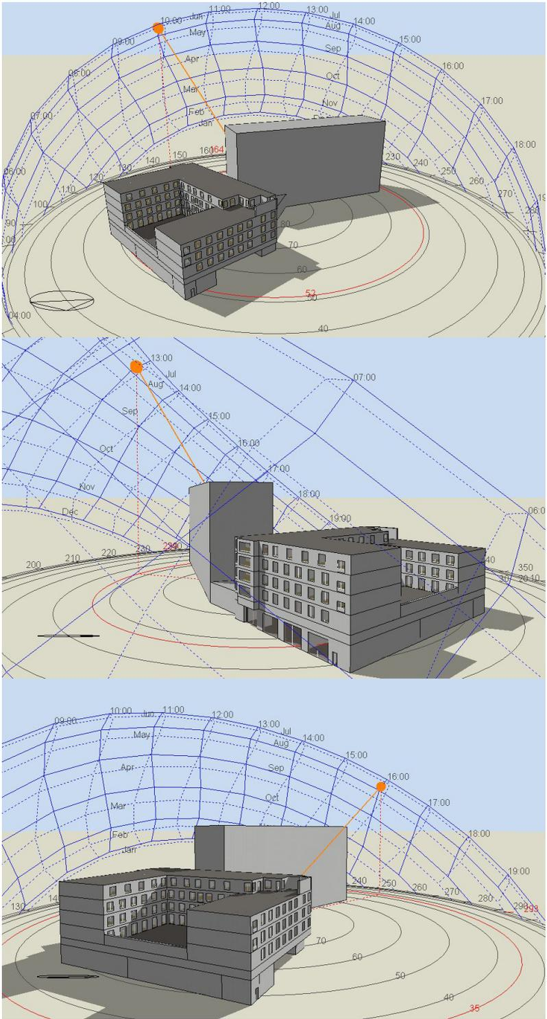
**Figure 9. Rendered view of the modelled building at 10am (top), 1pm (middle) and 4pm (bottom)**
