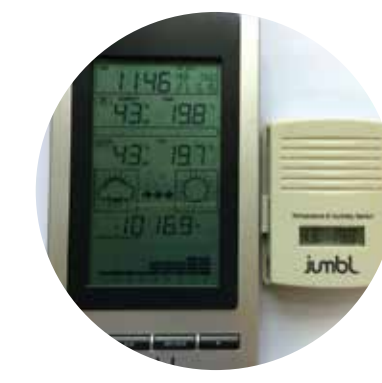
Electronic weather station Measures temperature, dew point, atmospheric pressure and humidity.
