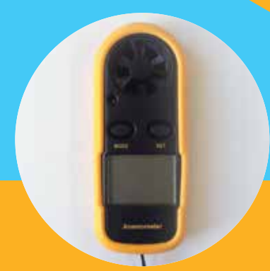
Anemometer Measures wind speed in mph.
