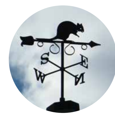
Wind vane Measures wind direction. It points in the direction in which the wind is blowing from. © Graham Lees, Flickr
