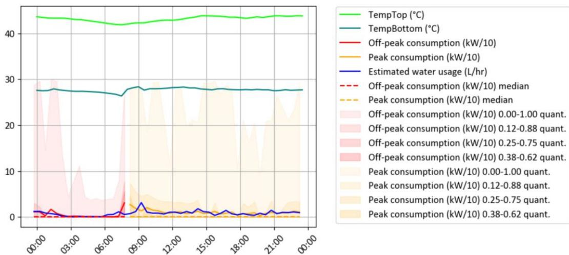
Figure 21: An incorrectly configured hot water device profile which appears to consume at all peak times.
