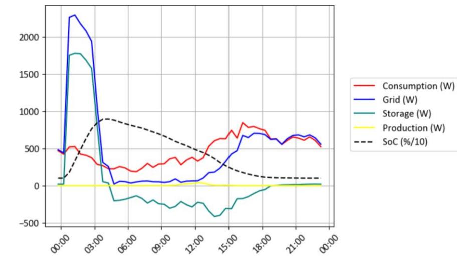
**Figure 5: The daily profile (81 days) of the single battery on the Octopus Go tariff. Coincidentally this device has the lowest PV output of the fleet.**
