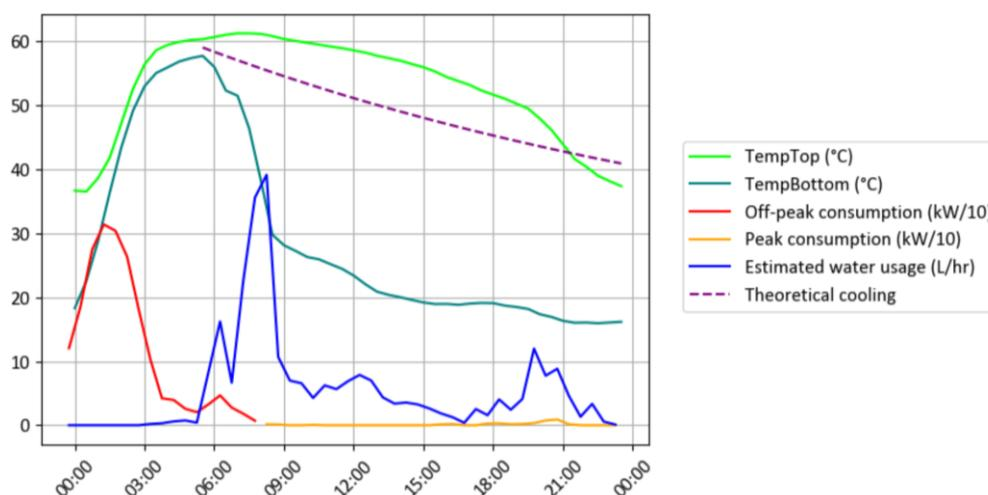
**Figure 22: A daily profile for a single hot water device, with the dashed purple line showing the predicted cooling without any water usage. The ambient temperature for this device is estimated at 23 degrees.**
