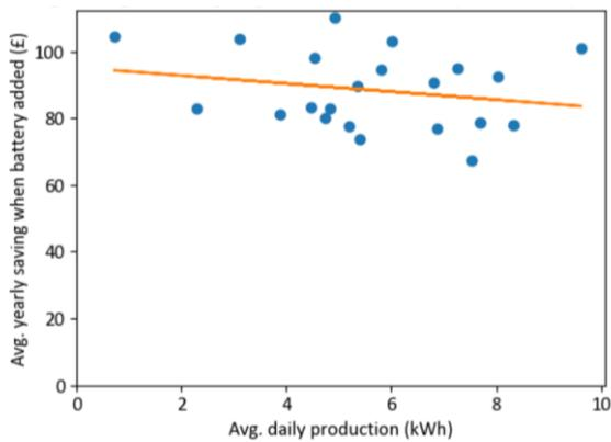
**Figure 29: Savings due to the battery on the Agile + Outgoing 2019 tariff against average daily production, showing no significant correlation ( $r=-0.22$ )**
