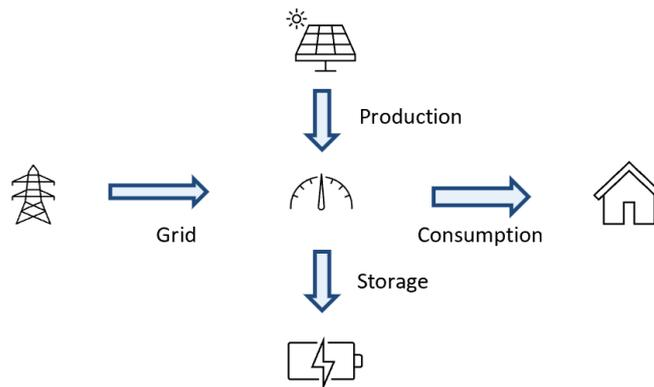
**Figure 2: Diagram of energy flows in a household with solar PV (top) and battery (bottom) installed and grid (left) and consumption (right) illustrated, indicating the terminology and sign convention in relation to the meter (centre) used in this report.**
