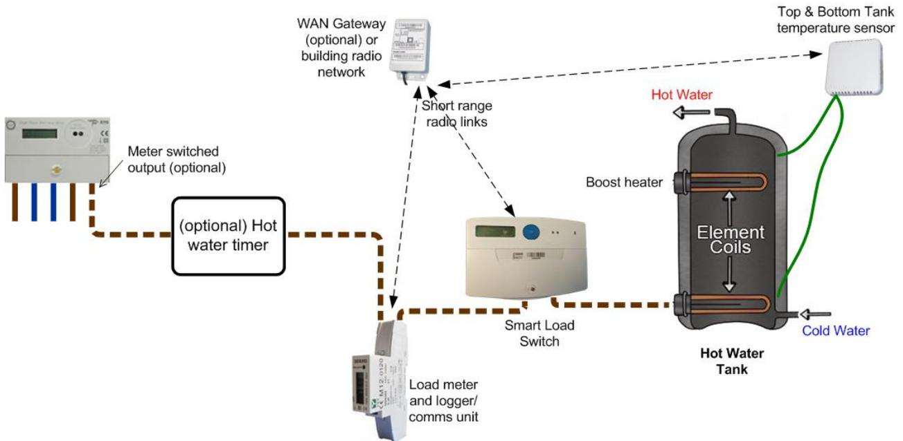
**Figure 3: A diagram of the Connected Response smart control and monitoring system attached to a ‘typical’ hot water tank; some existing electrical equipment such as the off-peak timer circuit is not shown.**
