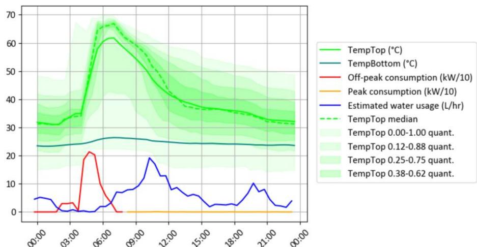
**Figure 19: A hot water tank which is apparently undersized.**
