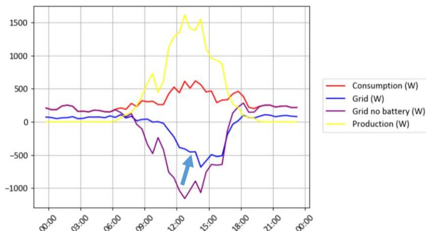
**Figure 38: Real battery behaviour on a single day (16/08/2021) with high PV production and low daytime prices, averaged over all devices, showing the reduction in grid export at times of solar peak for the battery case. Almost all batteries are optimised for a flat tariff.**
