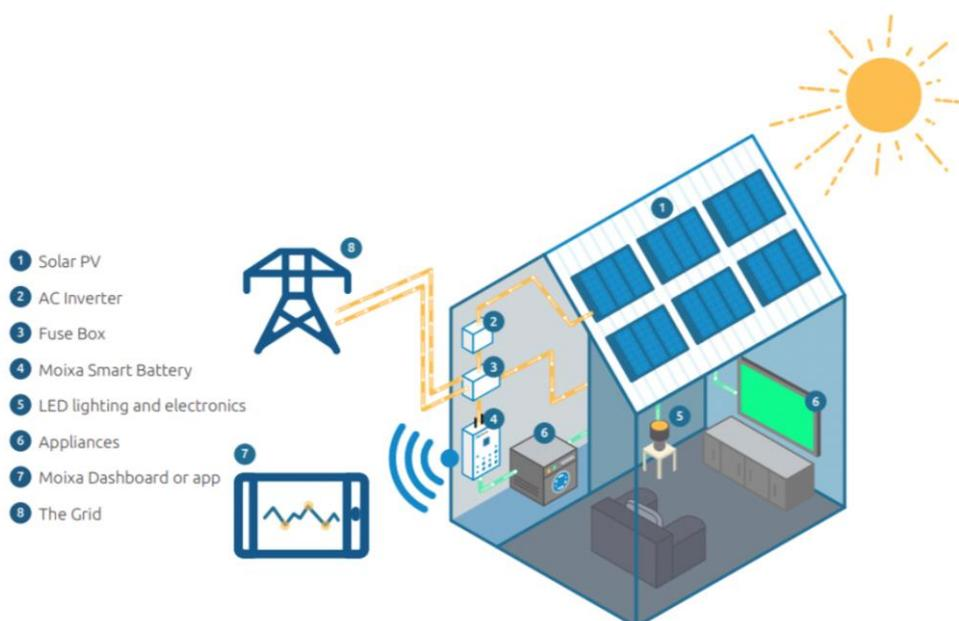
**Figure 1: Diagram of Moixa’s smart battery system installed in a house with PV panels.**
