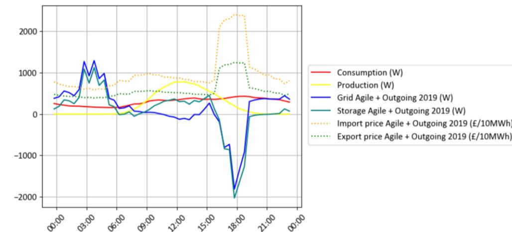
**Figure 26: The simulated battery behaviour responding to the Agile + Outgoing 2019 prices, averaged over all devices. The addition of the battery reduces the average cost on this tariff by £88/year down to just £44/year.**
