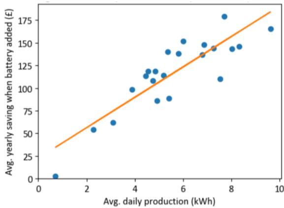
**Figure 27: Savings due to the battery on the Flat 18.4p tariff against average daily solar production, showing a strong correlation (Pearson's  $r = 0.87$ )**
