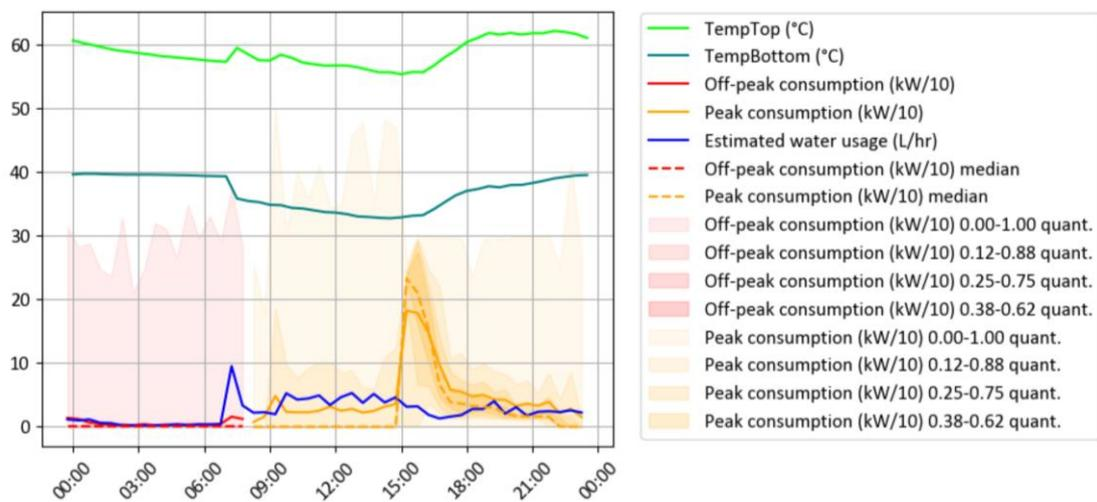
Figure 20: An incorrectly configured hot water device profile whose clock appears to be out of sync.
