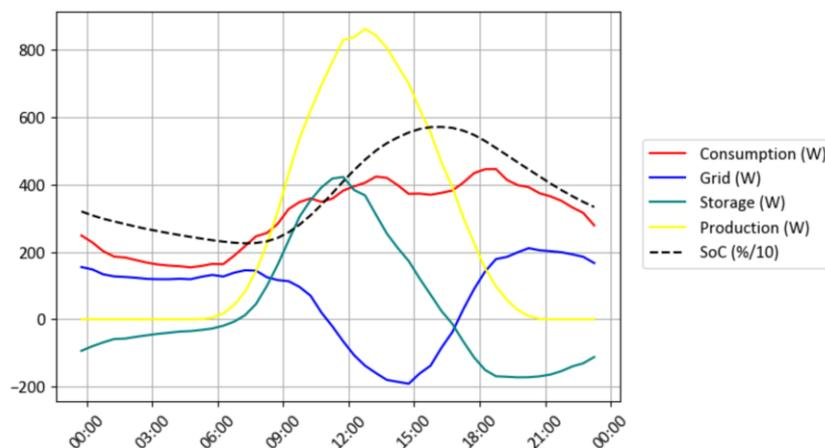
**Figure 4: The average daily profile of the 21 battery devices on flat tariffs over the whole trial period.**
