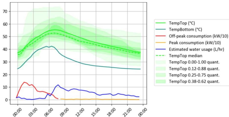
**Figure 18: The daily profile for the 14 well-understood hot water devices, with quartiles showing the variation between devices of the top temperature sensor.**
