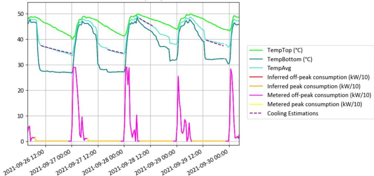
**Figure 47: The cooling estimations (dashed purple) superimposed on 4 days of data from a single hot water device. The estimations fit closely to the  $Temp_{Avg}$  line (midpoint of  $Temp_{top}$  and  $Temp_{bottom}$ ).**
