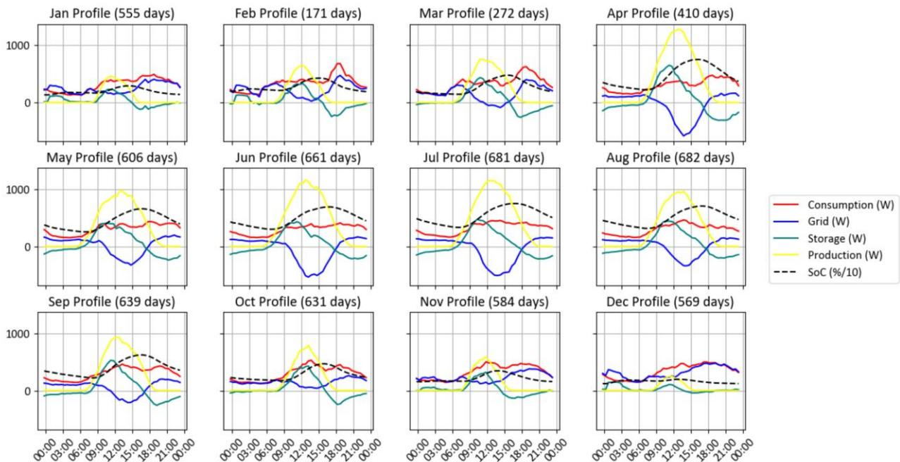
**Figure 8: Battery data segmented by month.**
