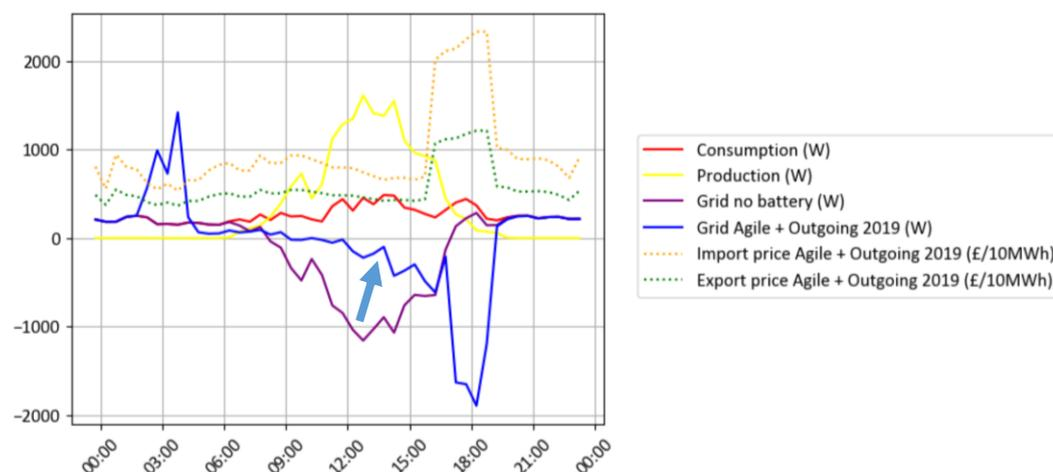
**Figure 39: Simulated behaviour on Agile Outgoing 2019 tariff on the same day (16/08/2021) with high PV production and low daytime prices, averaged over all devices, showing the reduction in grid export at times of solar peak for the battery case.**
