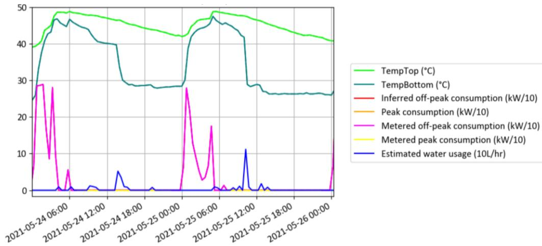
**Figure 9: A two-day excerpt from a hot water device which exhibits the ‘normal’ profile.**
