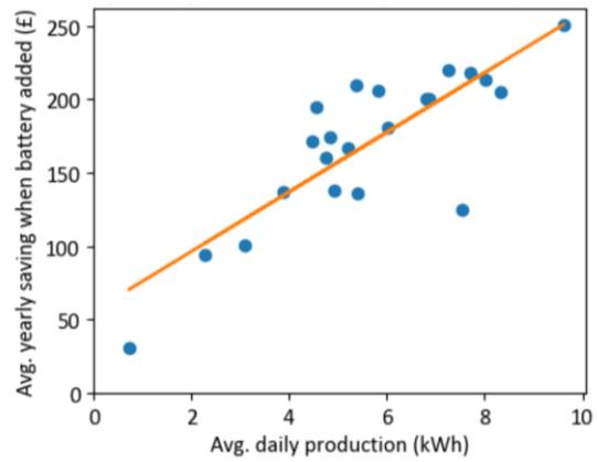
**Figure 28: Savings due to the battery on the Agile tariff against average daily solar production, showing a strong correlation ( $r=0.83$ )**
