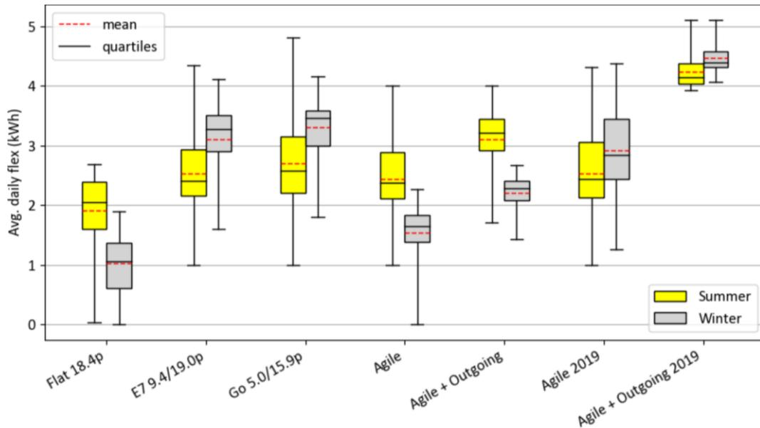
**Figure 35: The amount of ‘flexibility’, i.e. the average gross battery output per day, segmented by summer and winter, on various tariffs. The batteries all have a capacity of 4.8kWh.**
