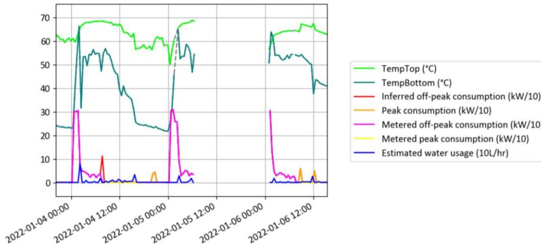
**Figure 10: A two-day excerpt from a hot water device with irregular and noisy data.**
