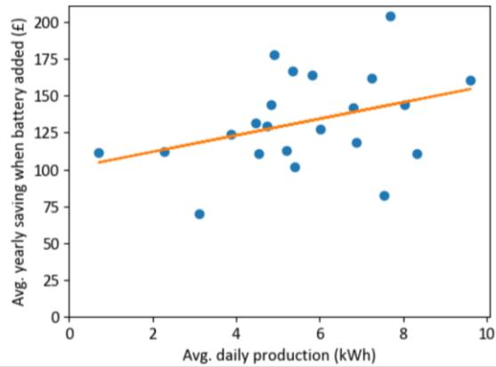
**Figure 30: Savings due to the battery on the Go 5.0/15.9p tariff against average daily production, showing a weak correlation ( $r=0.37$ )**
