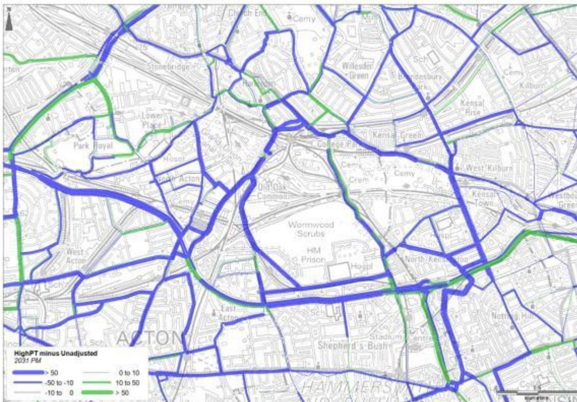
Figure 9-6: Traffic flows – Reduced Highway/ High PT Share scenario vs. Unadjusted scenario PM pk
