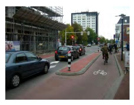
Dutch minor signal-controlled junction, in Assen. Motorists and cyclists move through the junction in separate phases
