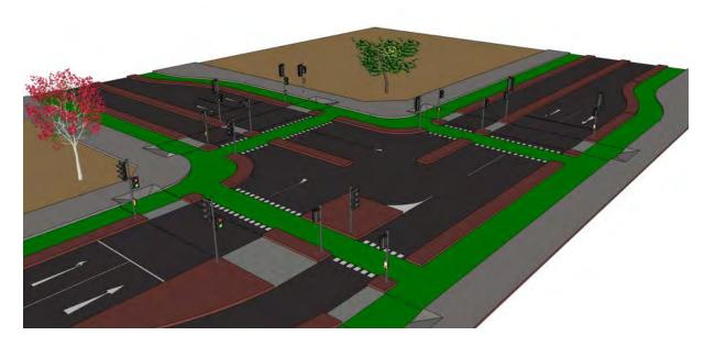
$3-D\ model\ of\ a\ possible\ UK\ traffic-controlled\ junction,\ with\ separate\ cycle\ tracks.\ Signal\ arrangements\ keep\ the\ movements\ of\ motor\ vehicles\ and\ cyclists\ separate.\ Courtesy\ of\ LCC\ Croydon\ Cycling\ Campaign$
