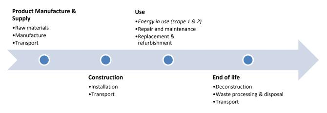
Figure 1.1: Building life cycle stages. All are considered as embodied emissions except the highlighted 'Energy in use' emissions. Source: Adapted from BS EN 15643-2:2011.
