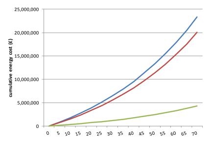
Figure 3.1: Cumulative energy costs for operating three equivalent commercial building designs (based on 2010 prices) Source: Best Foot Forward. The performance of the low carbon building is indicated with a green line.
