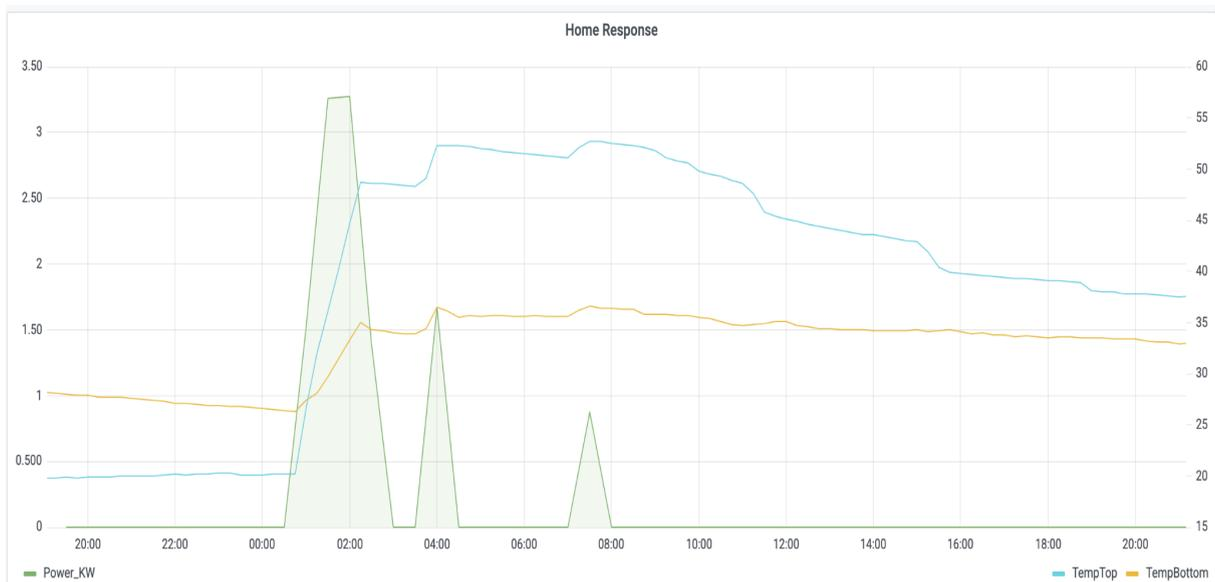
Figure 1. Typical energy and temperature profile of a domestic hot water heating system
