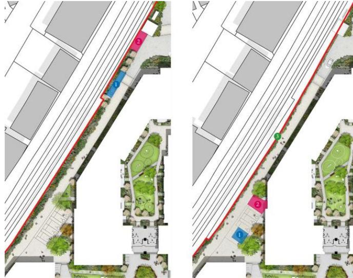
The July 2020 scheme incorporated 2 car club bays running perpendicular to the northwest boundary. Due to the changes to the site boundary, the parking layout has been amended, with the car club bays relocated adjacent to the concierge at the base of Block B. Two further spaces have been created to the west of Block C, resulting in loss of landscaping, as shown in Image 3 on the comparison plan extracts below:
