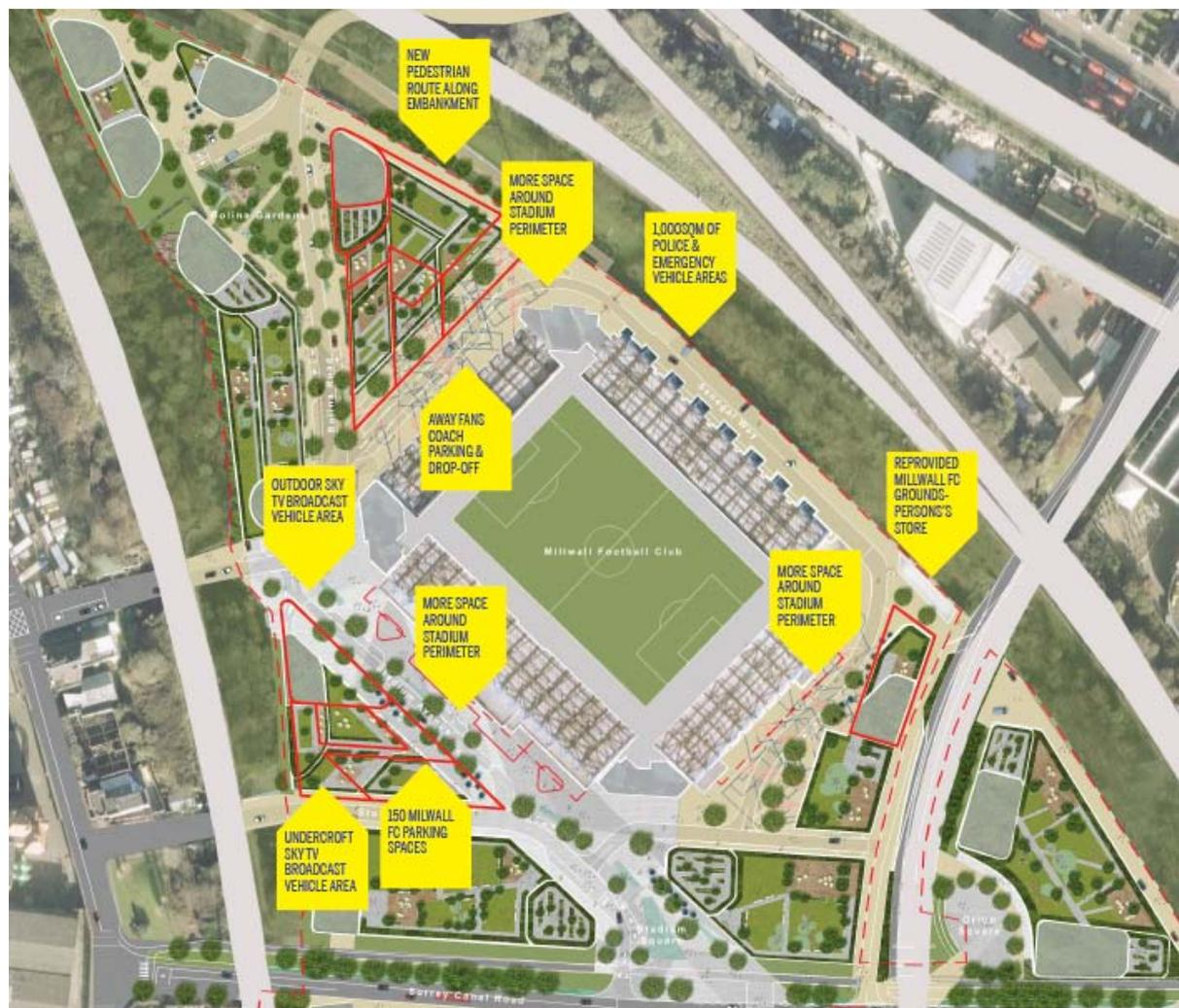
Figure 1: Alterations to the masterplan to accommodate the observations of Millwall FC and the Metropolitan Police. (Source: Applicant's design and access statement addendum).
