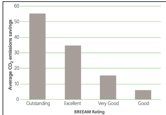
Figure 17: Average CO 2 emission saving for each type of rating compared to building regulation Part L 2010
