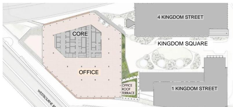
Figure 13: Schematic 1F plan, which shows the typical office floor plate.
