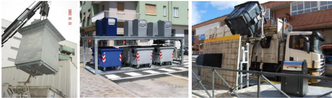
Figure 25: Examples of URS (left: crane lift system, middle: rear-loading hydraulic lift system, right: side-loading hydraulic lift system)
