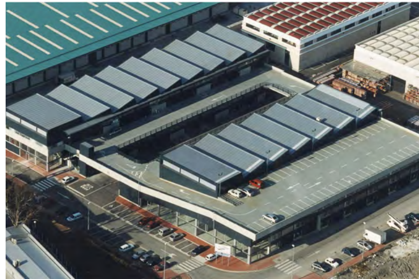
Belartza, Donostia-San Sebastian The stacking of smaller industrial types on upper floors enables a tighter site planning of ramps
