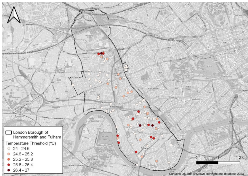
Figure 3-1 - Council housing properties at overheating risk defined by modelled temperature thresholds of internal temperature 3 .
