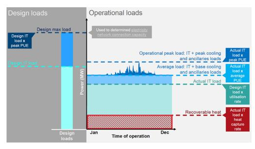
Fig 16. Loading profile of data centres. [Source: Arup Data Centre Energy Modelling]
