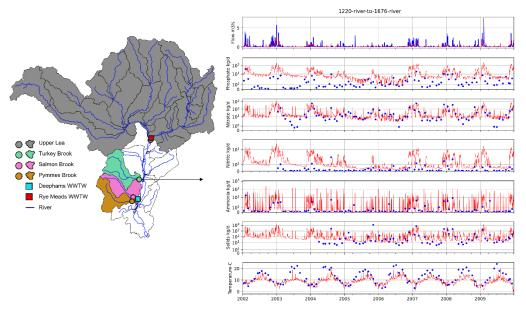
Figure D.21 shows simulation results for the Upper Lea at Feildes weir (flow) and further downstream for water quality. We see reasonable ammonia simulations and good phosphate simulations at the start of the timeseries but worsening throughout. We expect that the observed drop in phosphate amount that is not reflected in our simulations is due to the changing behaviour at Rye Meads WWTW (see following section).
