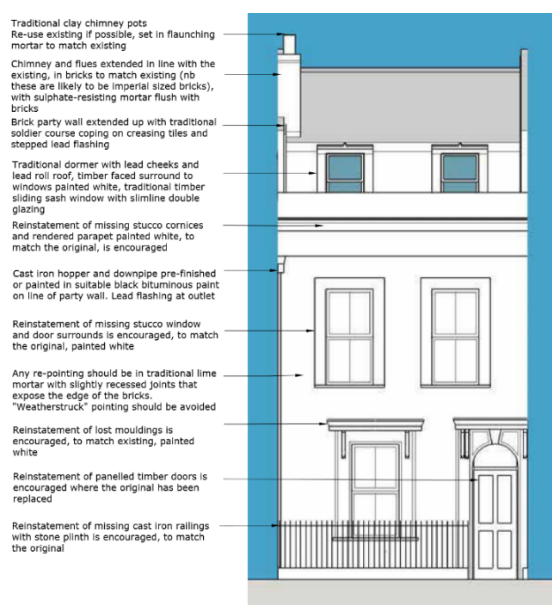
Figure A2.37 Architectural detailing that could form part of the planning conditions for an upward extension
