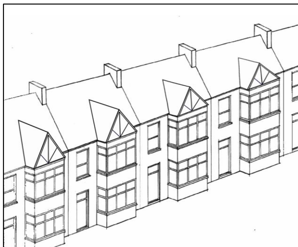
Figure A2.32 Inappropriate extension
