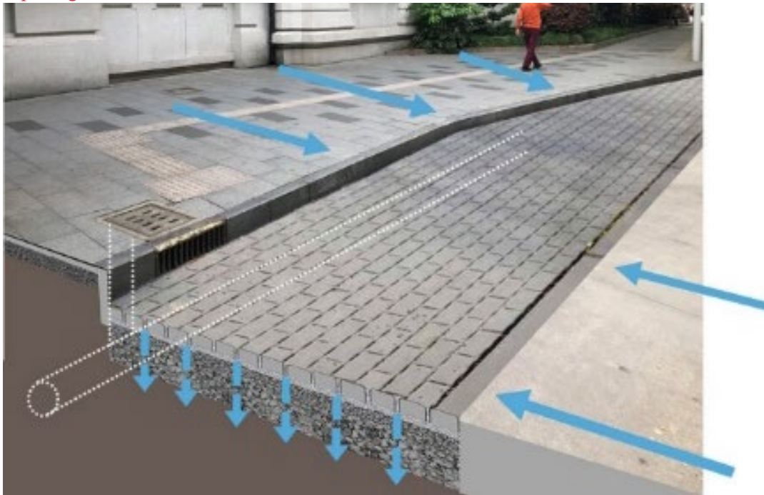
Figure 78: Example of permeable paving (Source: Arup).
