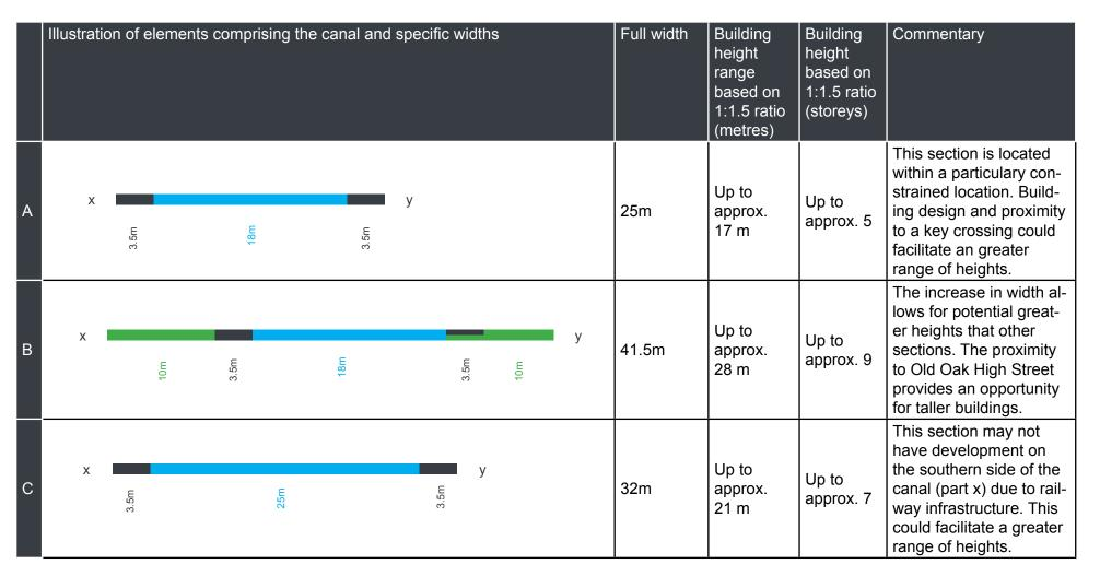
The above analysis demonstrates that the width of the Grand Union Canal will vary, responding to the width of the water space and adjacent uses and spaces. Consideration needs to be given to delivering a balanced approach to provide enclosure to spaces along the canal through building heights. Particularly, this will require building height policies to respond to the need to conserve and enhance Grand Union Canal Conservation Area and SINC designation and to support local legibility.
