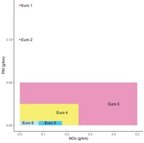
$\label{eq:Figure 2.5-Trends in Euro emission standards for NOx and PM for light duty diesels}$
