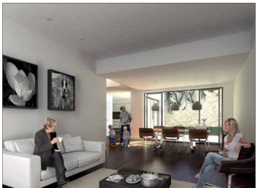
View across living area - changes in ceiling height define spaces within open-plan layout
