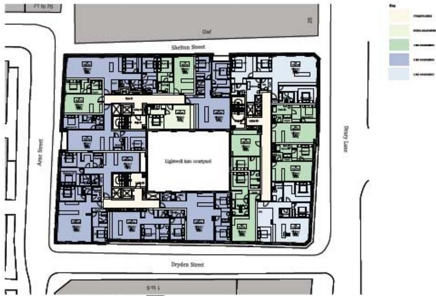
Proposed Typical Floor Plan (Third Floor) 1:200
