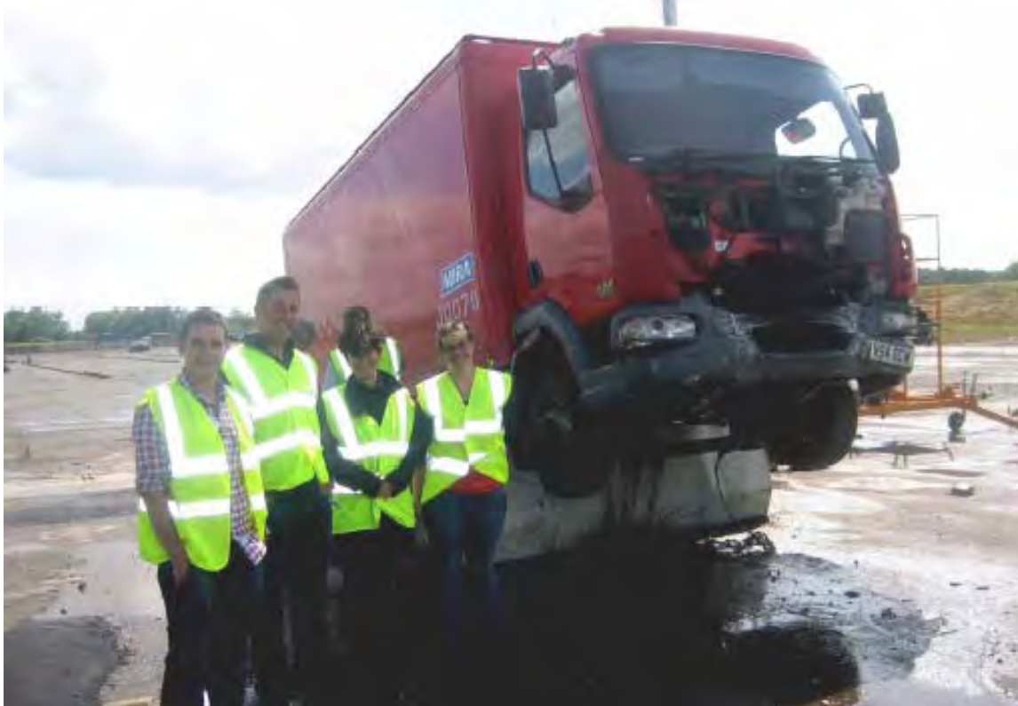
M15 Crash test of high security bench (7.5 tonnes, 48km/hr, 90 degree impact: 5.2m penetration)
