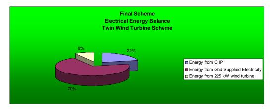
Using the single energy centre model of a 770kWe CHP and 2200kW biofueled plant, this combined with wind turbines would lead to a 26% renewable contribution on site. However, it can be seen that a combination of systems like this would be complex to build, operate and maintain with increased environmental impact and, as such, provides no real overall advantages.
