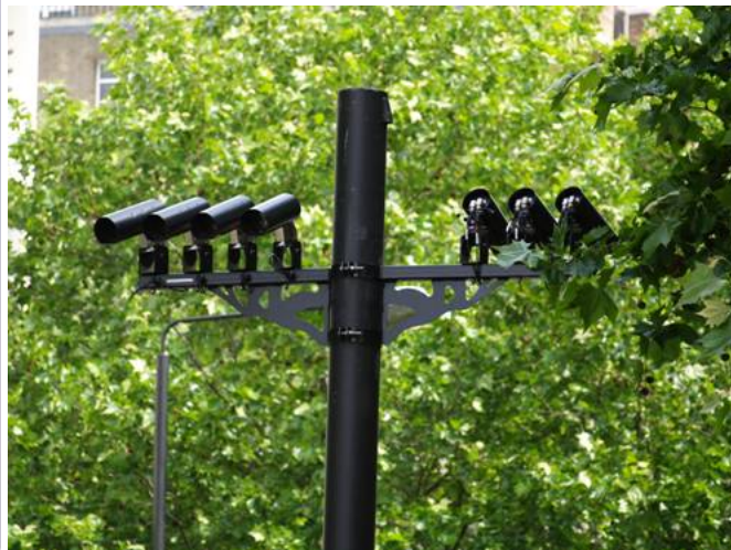
Typical Congestion Charging Western region Cameras (Smaller than in the original Congestion Charging region)
