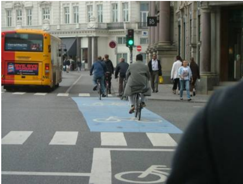
Figure 14: Copenhagen – use of colour to raise driver awareness and guide cyclists across junction
