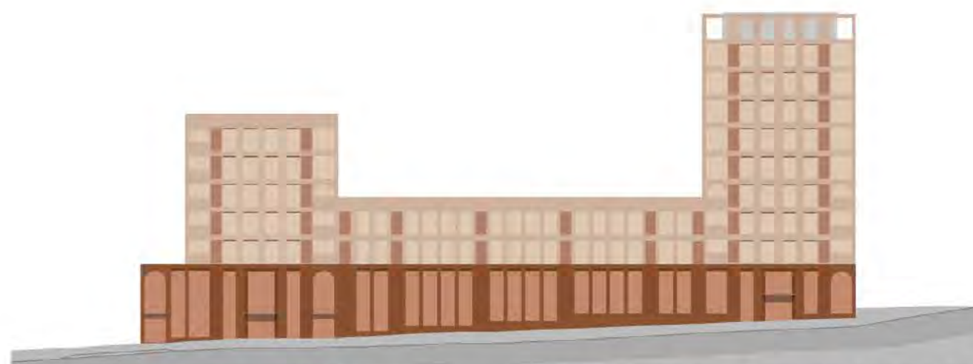
8. Lastly, wider piers are expressed through a textured surface, while the top of building is capped with an arched screen to hide the mechanical plant housing and to provide a distinct form to address the cityscale.
