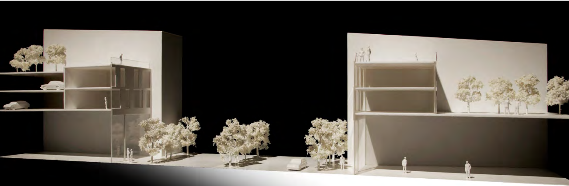
Sectional model looking west through typology 3 bisected by East Street, with large scale retail to the ground floor
