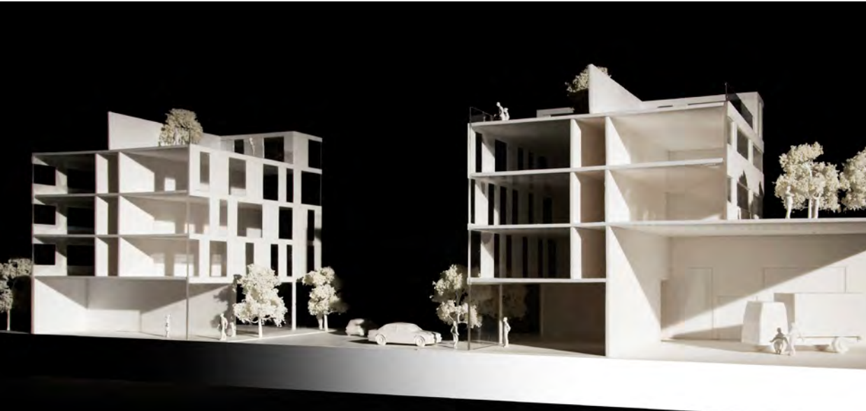
Sectional model through a side street to typology 3 looking north, showing retail units at the base, residential accommodation above and servicing / delivery bay to the rear, with raised courtyard above
