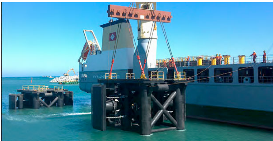
Figure 5: Dolphin designed for large lateral loads
