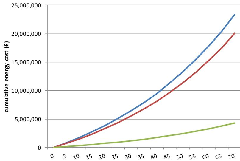
Figure 3.1: Cumulative energy costs for operating three equivalent commercial building designs (based on 2010 prices) Source: Best Foot Forward. The performance of the low carbon building is indicated with a green line.
