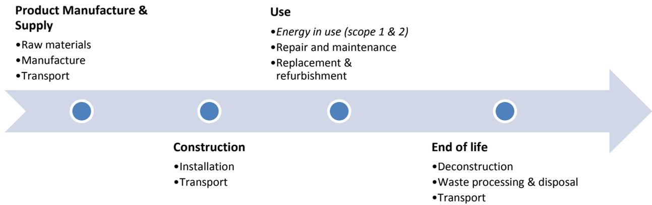
Figure 1.1: Building life cycle stages. All are considered as embodied emissions except the highlighted 'Energy in use' emissions. Source: Adapted from BS EN 15643-2:2011.
