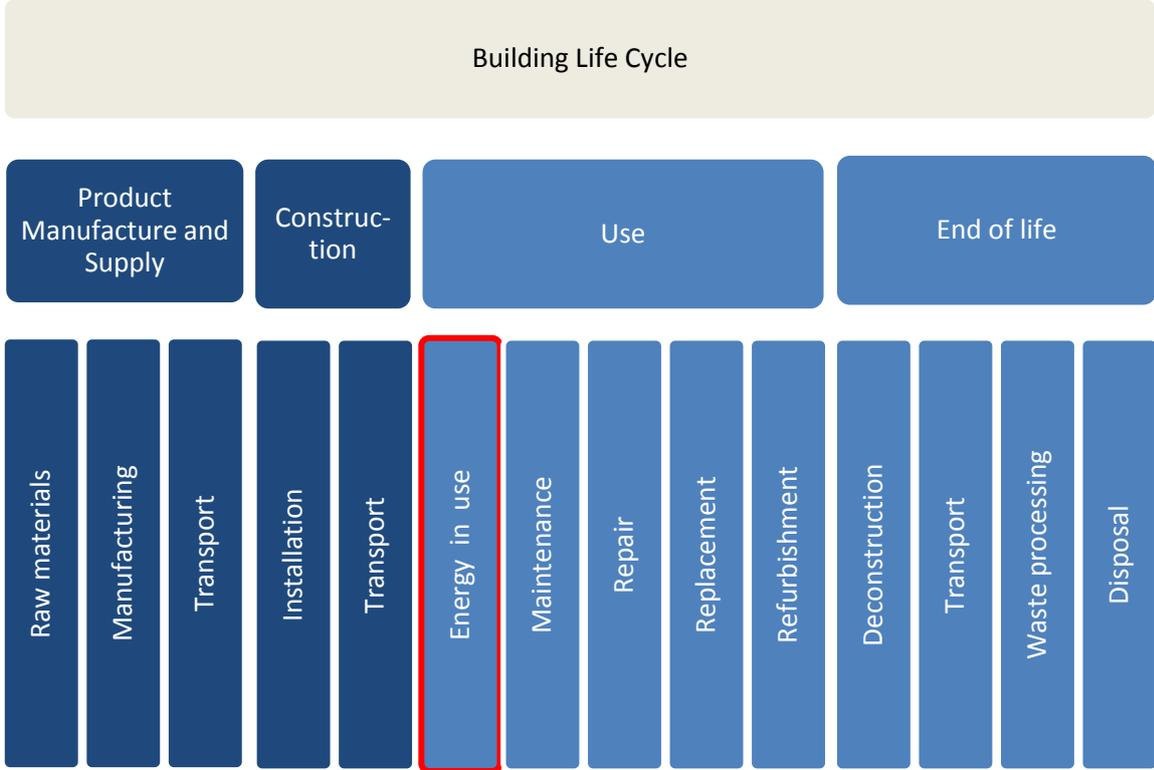
Figure 9.2: Building Life Cycle Stages. Adapted from BS EN 15978:2011. Note that all are considered embodied emissions except 'Energy in use'. Recommended stages are dark blue, discretionary stages are in lighter blue.
