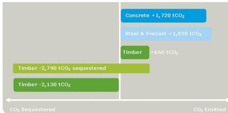
Carbon sequestration was modelled separately as well as with the cross-laminated timber frame. Even without sequestration considered, the timber frame has a much smaller embodied carbon footprint
