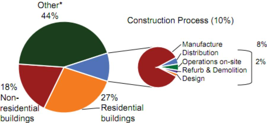
Figure 2.1: Proportion of total UK CO<sub>2</sub> emissions that construction can influence (split into in-use emissions for residential and non-residential buildings and construction-related emissions) Source: Department for Business Innovation and Skills.
