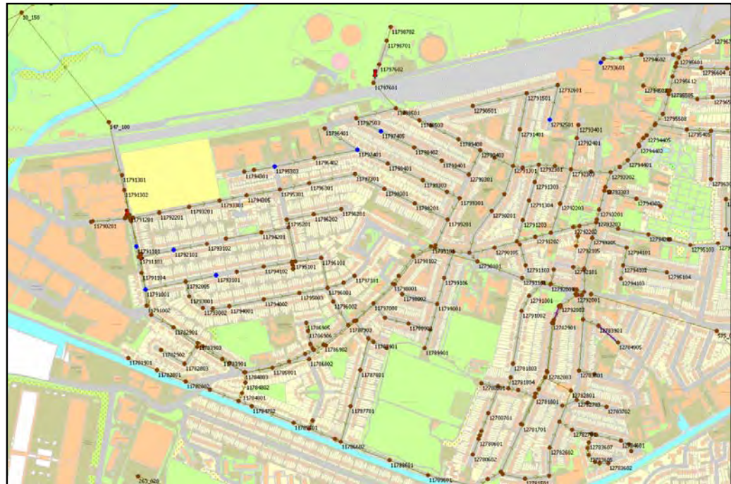
Figure 5: 1 in 2 year return period storm. Flooded nodes highlighted in blue.
