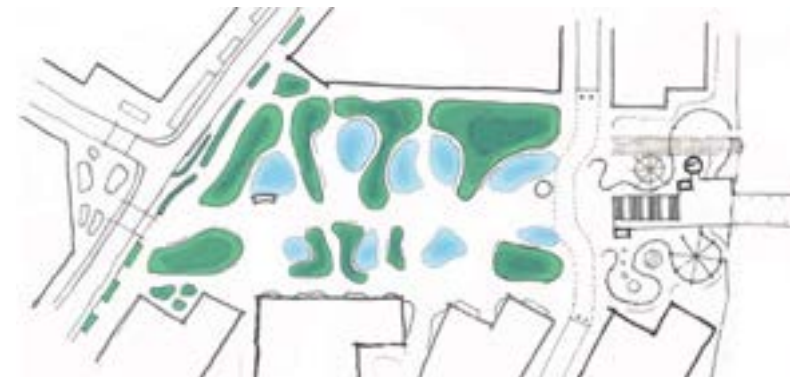
The topography of the park will be shaped by the need to attenuate stormwater storage
