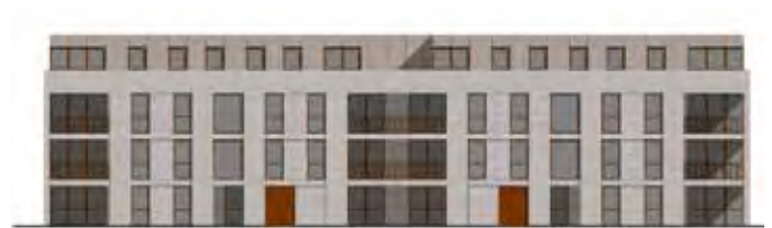
above: Proposed scheme- Calmer material palette complements, rather than competes with the landscape 3 storey brick façade with simple, rhythmic openings emphasises horizontal 'terrace' Set back roof storey limits sense of height opposite 2 storey viaduct wall
