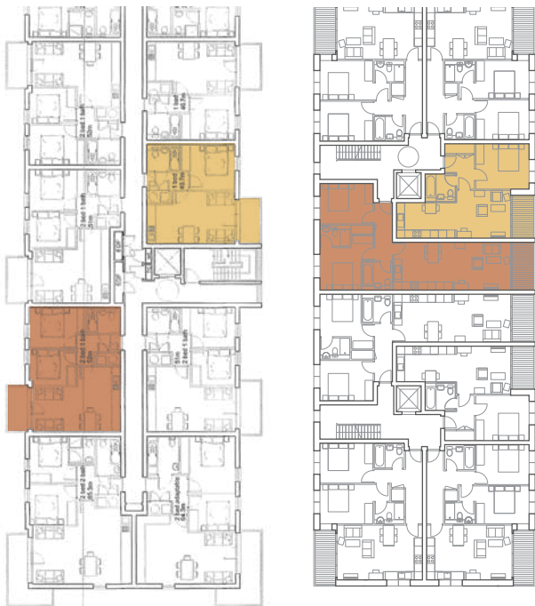
above left: Consented scheme- Small unit sizes, and an excess of single aspect units: 75% of units are single aspect 10 units to a single core (LHDG stipulates 8 maximum) 2 bed apartment only 51 m 2 GIA (10 m 2 below LHDG minimum) 1 bed apartment only 40 m 2 GIA (10 m 2 below LHDG minimum)
