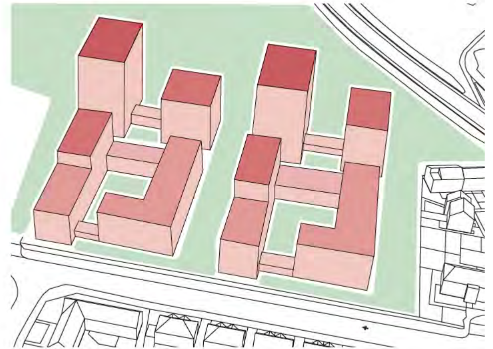
⑥ Height set to maximise daylight
