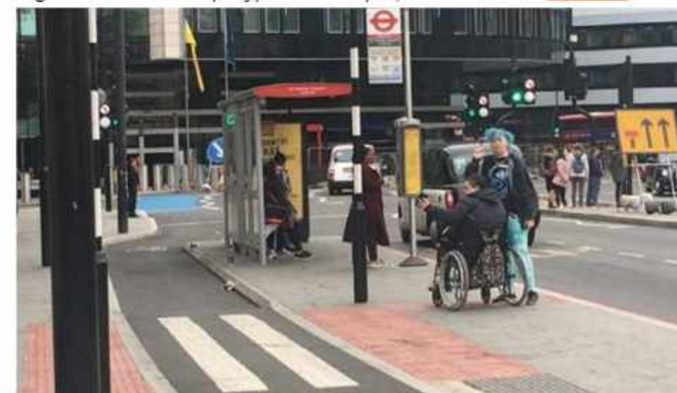
Figure 6.13 Bus stop bypass example, West-Sussex-London (2/39)
