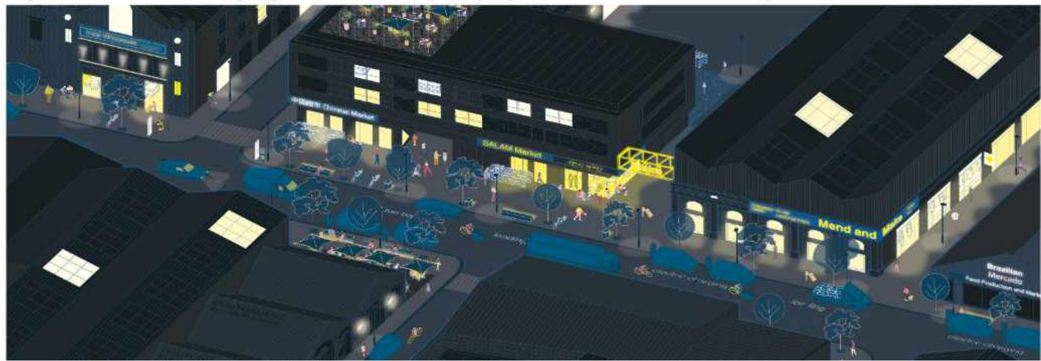
Figure 5.18 Illustration of how lighting, street furniture and planting help to create a safe environment along an industrial Local Street
