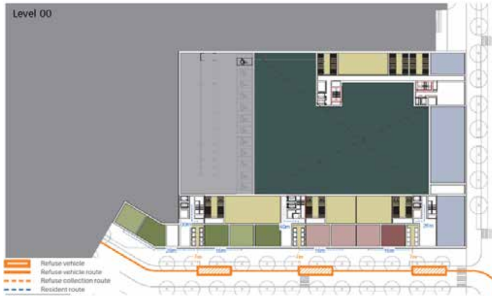
Plan 2: Distances travelled from the core (in orange) to the proposed bin store on levels 00 and 01.
