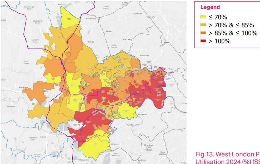
Fig 13. West London Primary Substation Peak Capacity Utilisation 2024 (%) (SSEN)
