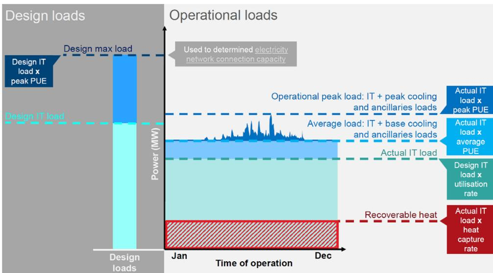
Fig 16. Loading profile of data centres. [Source: Arup Data Centre Energy Modelling]
