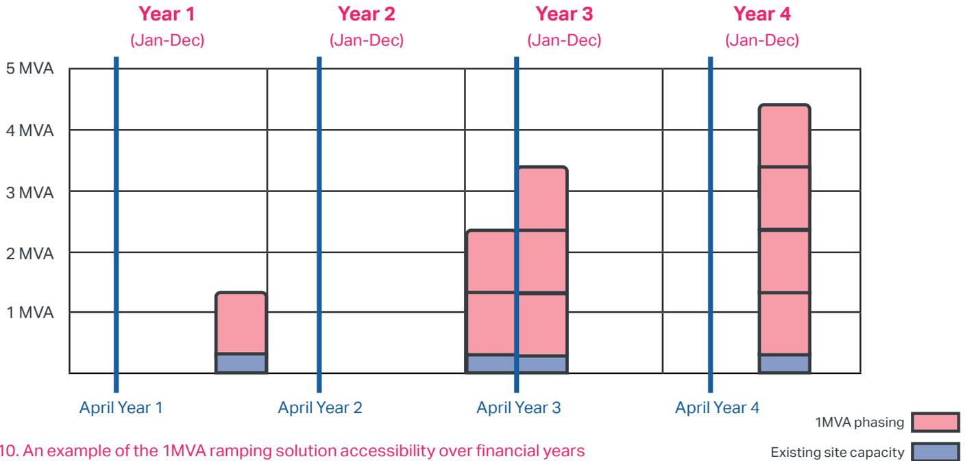
Fig 10. An example of the 1MVA ramping solution accessibility over financial years
